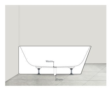
**8.** Apply silicone around the bath outline and allow it to set for a minimum of 24 hours.
